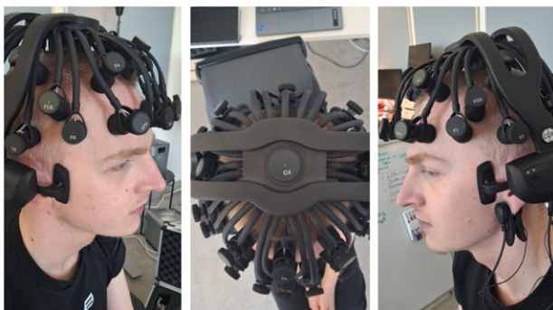
Figure 1. CGX Quick-32r EEG helmet placement on the head of the subject.
